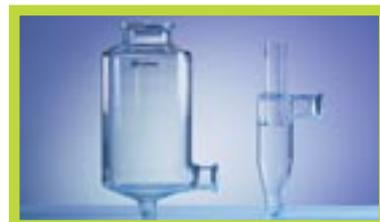
SD-Basic Cyclone and Drying Chamber
